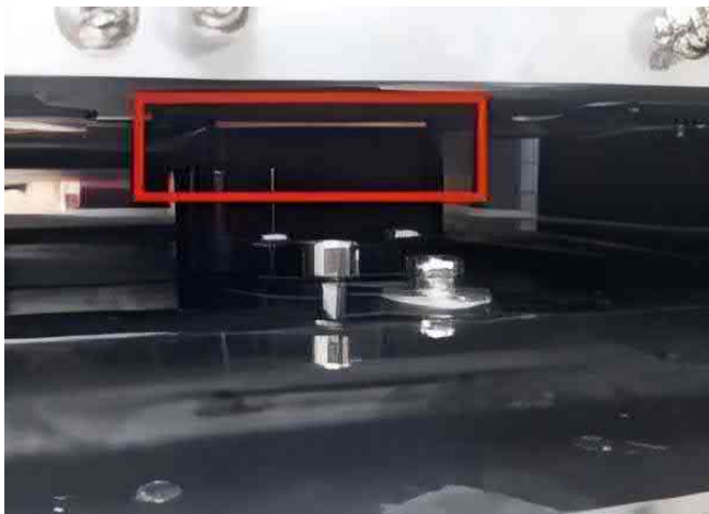
打印头表面和墨垫密封保湿 (Printhead surface and ink capping need to seal and moisturize)
