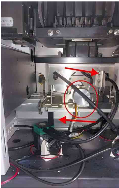
拧逆时针方向把墨栈复位好 Turn counterclockwise, place well the ink stack station
