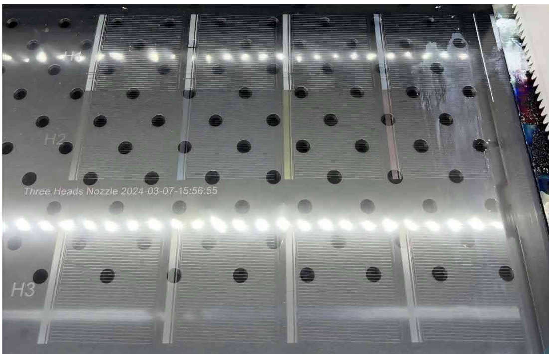
正常的测试条 Normal Test Strip ( all ink come out 100% and all color show in single line )
