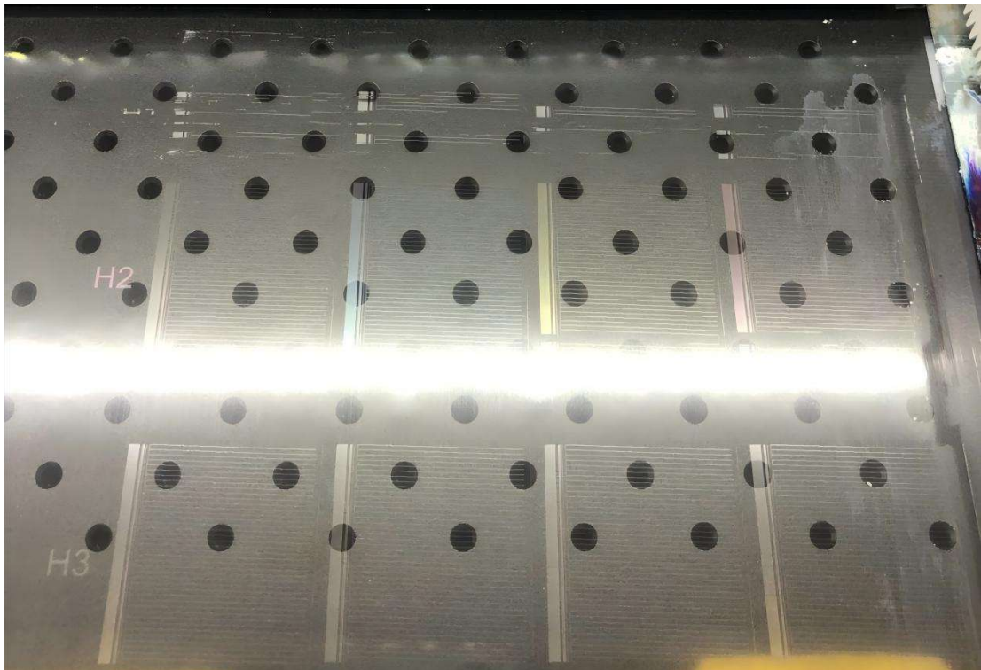
测试条断墨 Test Strip with problem ( ink not come out 100%, and all color not show in single line )
