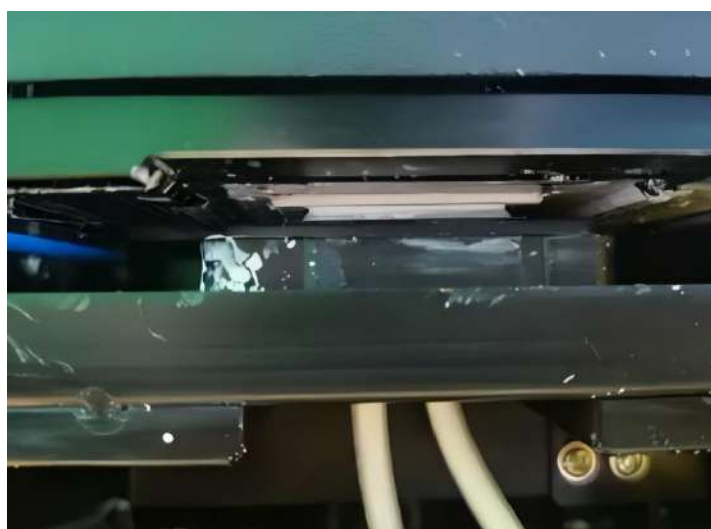
喷头居中并对齐墨垫（Best position, Center the print head on the ink pad ）
