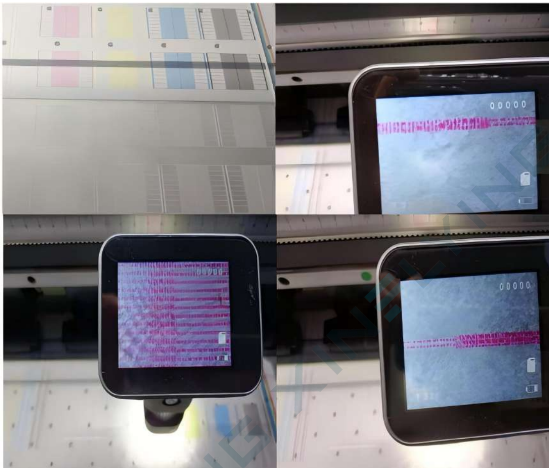
The figure below shows a properly calibrated vertical calibration chart and a red chromatic aberration chart.
