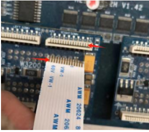
Correct(metal part to metal part)
