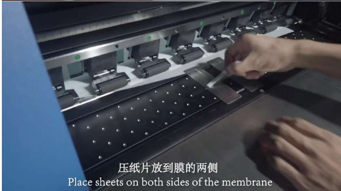
调节侧边的调节杆，将膜拉过来,压下调节杆 Adjust the adjustment bar on the side and pull the membrane over Press the regulator rod
