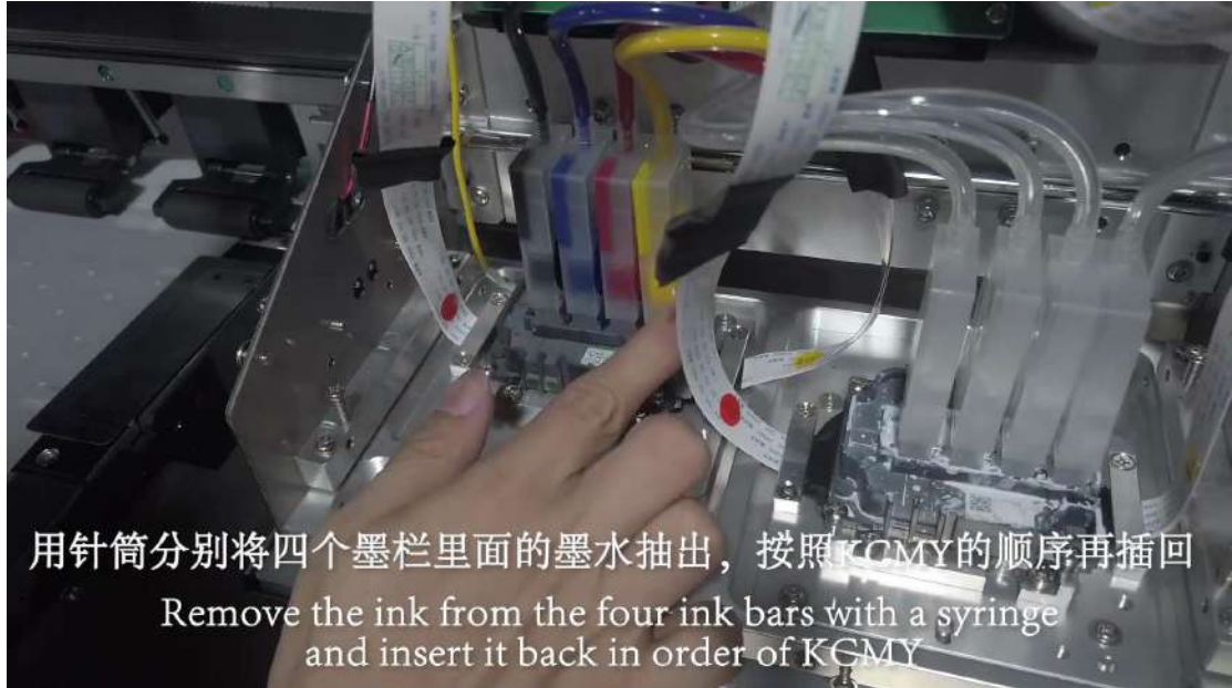
用针筒分别将四个墨栏里面的墨水抽出，按照KCMY的顺序再插回 Remove the ink from the four ink bars with a syringe and insert it back in order of KCMY
