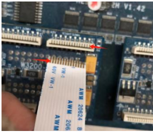
Correct(metal part to metal part)
